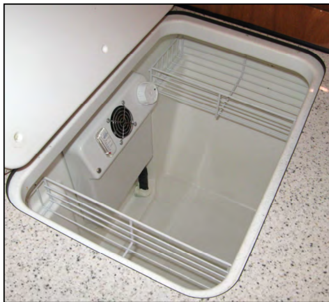
Hybrid Refrigerator Unit.
