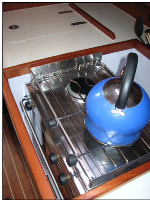
Stove with gimbals, safety bar and pot clamps.
